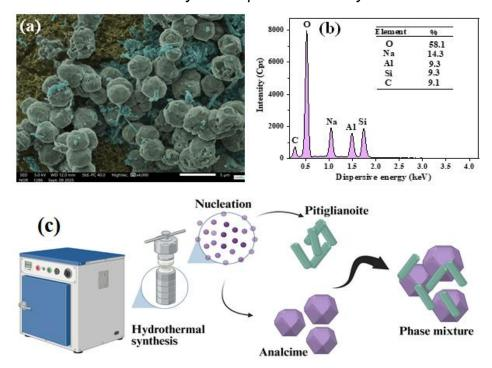
The energy peak corresponding to carbon observed in the EDX spectrum is related to the carbon tape used to fix the sample onto the metallic stub, which serves as the support during SEM analysis. Additionally, the elemental composition of the zeolitic matrix showed approximate proportions of 58.1% oxygen (O), 14.3% sodium (Na), 9.3% aluminum (Al), and 9.3% silicon (Si), values consistent with the typical stoichiometry of zeolitic structures.
